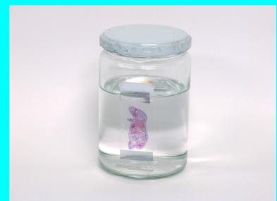
Fig. 3. Film-section on dissolving the adhesive in n-hexane.
